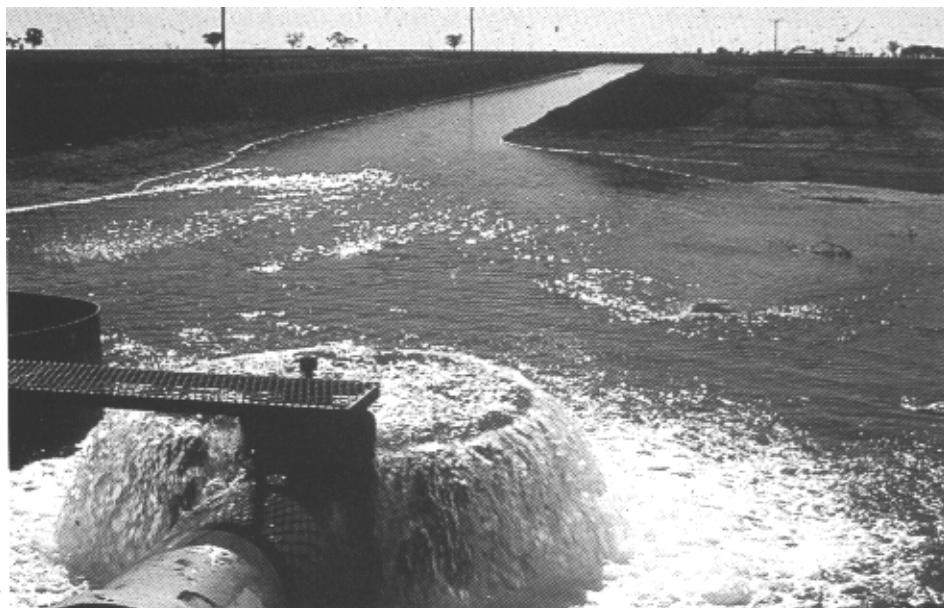
Pumping into an irrigation channel
