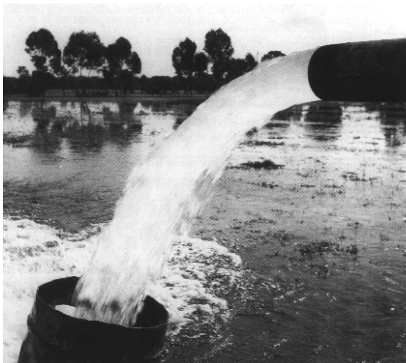
Pumping test on high yielding bore
