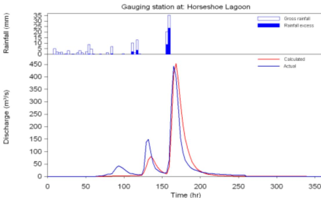
Figure A6.4: Plot of calibrated hydrograph
