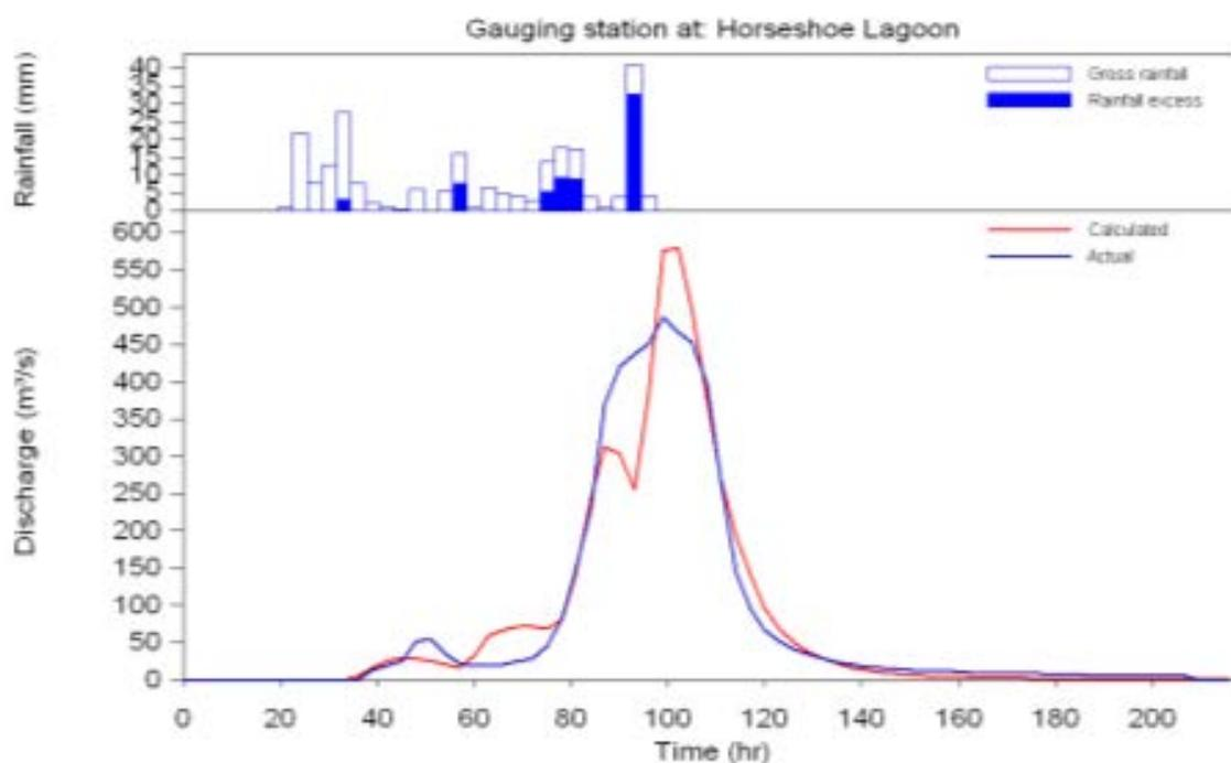
Figure A6.3: Hyetograph and calibrated hydrograph for the November 2011 flood event
