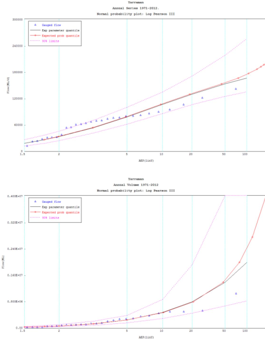
Figure A4.2: Comparison of flood frequency plots derived from peak discharges and flood volumes at Yarraman
