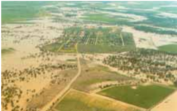
PLATE 13 - Ring Levee Protection
