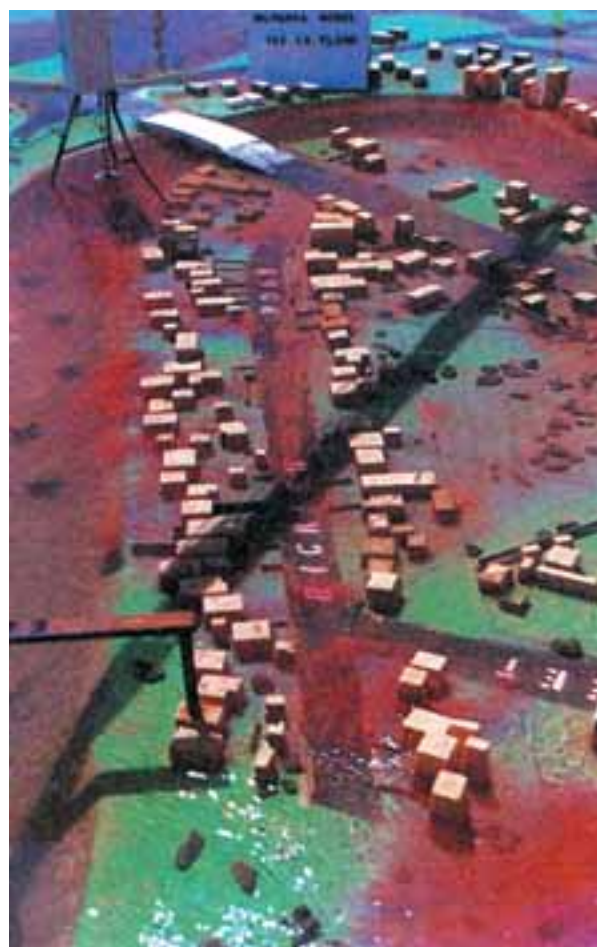
PLATE 8 - Physical Modelling of Flooding on the Georges River
